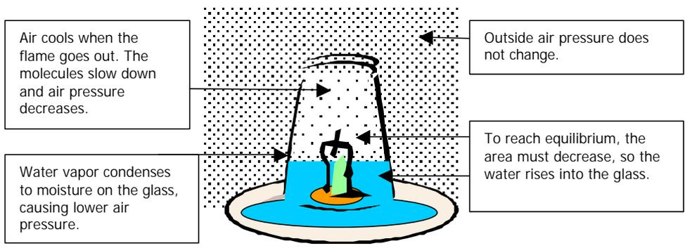
*The evaporation of the water to water vapor as the candle burns, and the cooling that occurs when the candle goes out, cause lower air pressure inside the glass than outside. The water is pushed into the glass until equilibrium is reached.)*
